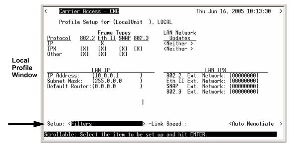
4. Press [CTRL A] to enable filters that have been defined. See the following sections on Defining Custom, Protocol and Address Filters.
